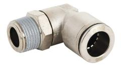
NITRA pneumatic push-to-connect fitting, elbow, rotating, nickelplated brass body, nickel-plated brass threads, thread sealant, (1) R3/8 male BSPT to (1) 1/2in push-to-connect. Package of 5.
