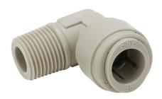
HydroMode potable water push-to-connect fitting, male, elbow, acetal body, acetal threads, (1) 1/2in tube to (1) 3/8in male NPT connection(s), NSF/ANSI 61. Package of 5.
