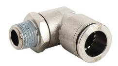
NITRA pneumatic push-to-connect fitting, elbow, rotating, nickel-plated brass body, nickel-plated brass threads, thread sealant, (1) R1/4 male BSPT to (1) 1/2in push-to-connect. Package of 5.
