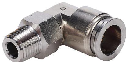
NITRA pneumatic push-to-connect fitting, elbow, rotating, 316 stainless steel body, 316 stainless steel threads, (1) 1/4in male NPT to (1) 1/2in push-to-connect.
