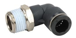
NITRA pneumatic push-to-connect fitting, elbow, rotating, thermoplastic (PBT) body, nickel-plated brass threads, thread sealant, (1) 1/2in male NPT to (1) 1/2in push-to-connect. Package of 5.
