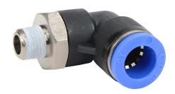
NITRA pneumatic push-to-connect fitting, elbow, rotating, thermoplastic (PBT) body, nickel-plated brass threads, thread sealant, (1) R1/8 male BSPT to (1) 10mm push-to-connect. Package of 5.
