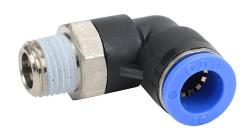
NITRA pneumatic push-to-connect fitting, elbow, rotating, thermoplastic (PBT) body, nickel-plated brass threads, thread sealant, (1) R1/4 male BSPT to (1) 10mm push-to-connect. Package of 5.
