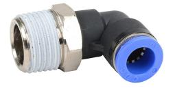
NITRA pneumatic push-to-connect fitting, elbow, rotating, thermoplastic (PBT) body, nickel-plated brass threads, thread sealant, (1) R1/2 male BSPT to (1) 10mm push-to-connect. Package of 5.
