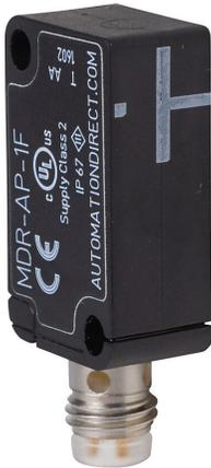
AutomationDirect magnetic proximity sensor, rectangular, 10.2 x 36.8 x 16mm body, polybutylene terephthalate housing, PNP, N.O. output, 60mm sensing distance, flush, 5 kHz switching frequency, IP67, 3-pin M8 quick-disconnect.
