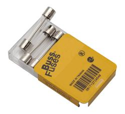
Bussmann fuse, MDL series, small dimension, time-delay, 8A, 250 VAC, glass tube. Package of 5. Supplemental, electronic protection applications. Manufacturer part number: MDL-8-R.
