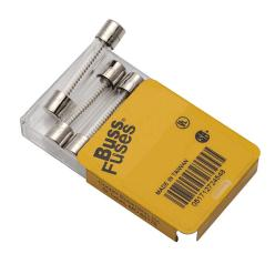
Bussmann fuse, MDL series, small dimension, time-delay, 15A, 32 VAC, glass tube. Package of 5. Supplemental, electronic protection applications. Manufacturer part number: MDL-15-R.
