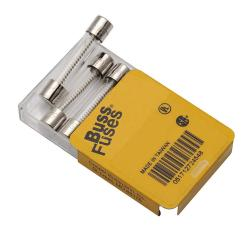
Bussmann fuse, MDL series, small dimension, time-delay, 1.5A, 250 VAC, glass tube. Package of 5. Supplemental, electronic protection applications. Manufacturer part number: MDL-1-1/2-R.
