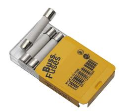
Bussmann fuse, MDA series, small dimension, time-delay, 3A, 250 VAC, ceramic tube. Package of 5. Supplemental, electronic protection applications. Manufacturer part number: MDA-3-R.
