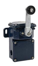
Schmersal heavy duty limit switch, side rotary lever with plastic roller, (1) N.O./(1) N.C. contact(s), snap action, 122mm hole spacing, cast iron, (2) M25  $\times$  1.5 cable entry.
