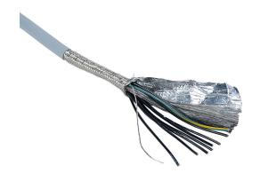
Southwire flexible control cable, shielded, 9 conductors (includes ground), 18 AWG, bare copper, PVC/Nylon conductor insulation material, black with white numbers and green/yellow ground, TPE jacket, gray, cut to length.
