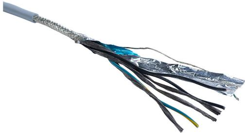
Southwire flexible control cable, shielded, 3 conductors (includes ground), 18 AWG, bare copper, PVC/Nylon conductor insulation material, black with white numbers and green/yellow ground, TPE jacket, gray, cut to length.
