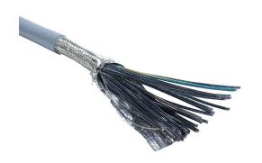
Southwire flexible control cable, shielded, 25 conductors (includes ground), 18 AWG, bare copper, PVC/Nylon conductor insulation material, black with white numbers and green/yellow ground, TPE jacket, gray, cut to length.
