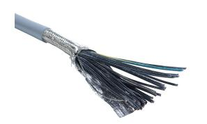
Southwire flexible control cable, shielded, 25 conductors (includes ground), 18 AWG, bare copper, PVC/Nylon conductor insulation material, black with white numbers and green/yellow ground, TPE jacket, gray, cut to length.
