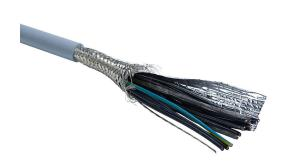
Southwire flexible control cable, shielded, 12 conductors (includes ground), 18 AWG, bare copper, PVC/Nylon conductor insulation material, black with white numbers and green/yellow ground, TPE jacket, gray, cut to length.
