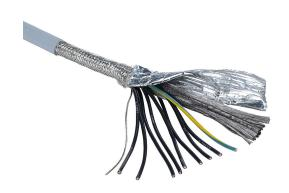
Southwire flexible control cable, shielded, 9 conductors (includes ground), 16 AWG, bare copper, PVC/Nylon conductor insulation material, black with white numbers and green/yellow ground, TPE jacket, gray, cut to length.
