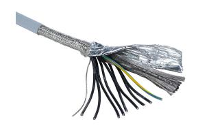
Southwire flexible control cable, shielded, 9 conductors (includes ground), 16 AWG, bare copper, PVC/Nylon conductor insulation material, black with white numbers and green/yellow ground, TPE jacket, gray, cut to length.
