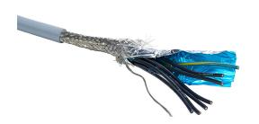
Southwire flexible control cable, shielded, 7 conductors (includes ground), 16 AWG, bare copper, PVC/Nylon conductor insulation material, black with white numbers and green/yellow ground, TPE jacket, gray, cut to length.
