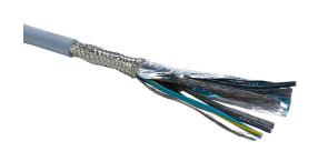
Southwire flexible control cable, shielded, 3 conductors (includes ground), 16 AWG, bare copper, PVC/Nylon conductor insulation material, black with white numbers and green/yellow ground, TPE jacket, gray, cut to length.
