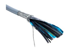
Southwire flexible control cable, shielded, 25 conductors (includes ground), 16 AWG, bare copper, PVC/Nylon conductor insulation material, black with white numbers and green/yellow ground, TPE jacket, gray, cut to length.
