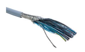
Southwire flexible control cable, shielded, 7 conductors (includes ground), 14 AWG, bare copper, PVC/Nylon conductor insulation material, black with white numbers and green/yellow ground, TPE jacket, gray, cut to length.
