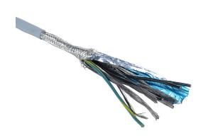
Southwire flexible control cable, shielded, 4 conductors (includes ground), 14 AWG, bare copper, PVC/Nylon conductor insulation material, black with white numbers and green/yellow ground, TPE jacket, gray, cut to length.
