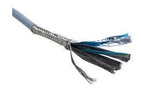
Southwire flexible control cable, shielded, 3 conductors (includes ground), 14 AWG, bare copper, PVC/Nylon conductor insulation material, black with white numbers and green/yellow ground, TPE jacket, gray, cut to length.
