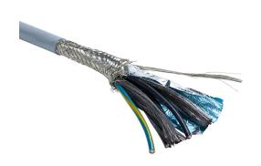
Southwire flexible control cable, shielded, 4 conductors (includes ground), 12 AWG, bare copper, PVC/Nylon conductor insulation material, black with white numbers and green/yellow ground, TPE jacket, gray, cut to length.
