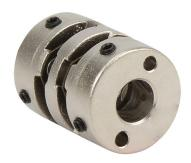
AutomationDirect encoder coupling, 8mm to 1/4in bore, aluminum alloy body, setscrew. For use with Koyo TRD-N/NA and TRDA-2E series encoders.
