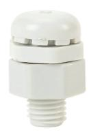
Bimed pressure relief vent plug, M6 x 0.75mm thread type, polyamide, light gray, 133 mL/min @ 70 mBar (1 psi), IP67 IP68 IP69K. Package of 2.
