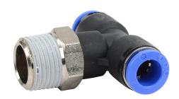
NITRA pneumatic push-to-connect fitting, male, branch tee, rotating, thermoplastic (PBT) body, nickel-plated brass threads, (2) 5/16in (8mm) tube to R3/8 BSPT connection(s). Package of 5.
