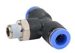
NITRA pneumatic push-to-connect fitting, branch tee, rotating, thermoplastic (PBT) body, nickel-plated brass threads, thread sealant, (1) R1/8 male BSPT to (2) 5/16in (8mm) push-to-connect. Package of 5.
