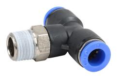
NITRA pneumatic push-to-connect fitting, branch tee, rotating, thermoplastic (PBT) body, nickel-plated brass threads, thread sealant, (1) R1/4 male BSPT to (2) 5/16in (8mm) push-to-connect. Package of 5.
