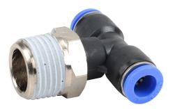
NITRA pneumatic push-to-connect fitting, branch tee, rotating, thermoplastic (PBT) body, nickel-plated brass threads, thread sealant, (1) R1/2 male BSPT to (2) 5/16in (8mm) push-to-connect. Package of 5.
