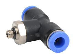
NITRA pneumatic push-to-connect fitting, branch tee, rotating, thermoplastic (PBT) body, nickel-plated brass threads, thread sealant, (1) M5  $\times$  0.8 male ISO to (2) 6mm push-to-connect. Package of 5.
