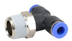
NITRA pneumatic push-to-connect fitting, male, branch tee, rotating, thermoplastic (PBT) body, nickel-plated brass threads, (2) 6mm tube to R3/8 BSPT connection(s). Package of 5.
