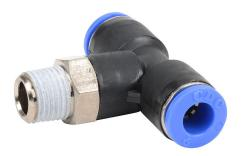
NITRA pneumatic push-to-connect fitting, branch tee, rotating, thermoplastic (PBT) body, nickel-plated brass threads, thread sealant, (1) R1/8 male BSPT to (2) 6mm push-to-connect. Package of 5.
