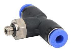
NITRA pneumatic push-to-connect fitting, branch tee, rotating, thermoplastic (PBT) body, nickel-plated brass threads, thread sealant, (1) M5 x 0.8 male ISO to (2) 5/32in (4mm) push-to-connect. Package of 5.
