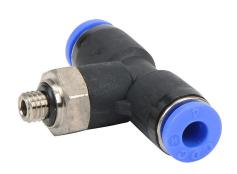
NITRA pneumatic push-to-connect fitting, male, branch tee, rotating, thermoplastic (PBT) body, nickel-plated brass threads, (2) 5/32in (4mm) tube to M5 X 0.8 threaded connection(s). Package of 5.
