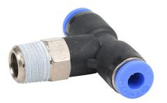
NITRA pneumatic push-to-connect fitting, branch tee, rotating, thermoplastic (PBT) body, nickel-plated brass threads, thread sealant, (1) R1/8 male BSPT to (2) 5/32in (4mm) push-to-connect. Package of 5.
