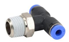
NITRA pneumatic push-to-connect fitting, branch tee, rotating, thermoplastic (PBT) body, nickel-plated brass threads, thread sealant, (1) R1/4 male BSPT to (2) 5/32in (4mm) push-to-connect. Package of 5.
