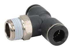
NITRA pneumatic push-to-connect fitting, branch tee, rotating, thermoplastic (PBT) body, nickel-plated brass threads, thread sealant, (2) 3/8in push-to-connect to (1) 3/8in male NPT. Package of 5.
