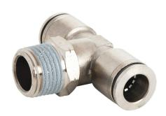
NITRA pneumatic push-to-connect fitting, male, branch tee, rotating, nickel-plated brass body, nickel-plated brass threads, thread sealant, (2) 3/8in push-to-connect to 3/8in NPT. Package of 5.
