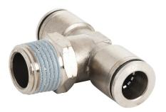
NITRA pneumatic push-to-connect fitting, branch tee, rotating, nickel-plated brass body, nickel-plated brass threads, thread sealant, (2) 3/8in push-to-connect to (1) 3/8in male NPT. Package of 5.
