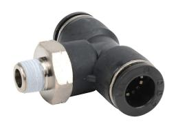
NITRA pneumatic push-to-connect fitting, branch tee, rotating, thermoplastic (PBT) body, nickel-plated brass threads, thread sealant, (2) 3/8in push-to-connect to (1) 1/8in male NPT. Package of 5.
