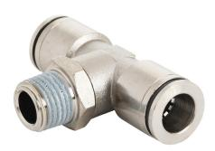
NITRA pneumatic push-to-connect fitting, branch tee, rotating, nickel-plated brass body, nickel-plated brass threads, thread sealant, (1) R1/4 male BSPT to (2) 3/8in push-to-connect. Package of 5.
