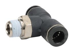
NITRA pneumatic push-to-connect fitting, branch tee, rotating, thermoplastic (PBT) body, nickel-plated brass threads, thread sealant, (1) 1/4in male NPT to (2) 3/8in push-to-connect. Package of 5.
