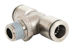
NITRA pneumatic push-to-connect fitting, male, branch tee, rotating, nickel-plated brass body, nickel-plated brass threads, thread sealant, (2) 3/8in push-to-connect to 1/4in NPT. Package of 5.
