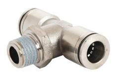
NITRA pneumatic push-to-connect fitting, branch tee, rotating, nickel-plated brass body, nickel-plated brass threads, thread sealant, (1) 1/4in male NPT to (2) 3/8in push-to-connect. Package of 5.
