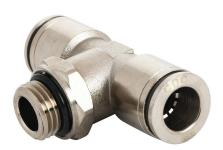
NITRA pneumatic push-to-connect fitting, male, branch tee, rotating, nickel-plated brass body, nickel-plated brass threads, thread sealant, (2) 3/8in push-to-connect to G1/4 BSPP. Package of 5.
