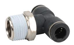
NITRA pneumatic push-to-connect fitting, branch tee, rotating, thermoplastic (PBT) body, nickel-plated brass threads, thread sealant, (1) 1/2in male NPT to (2) 3/8in push-to-connect. Package of 5.
