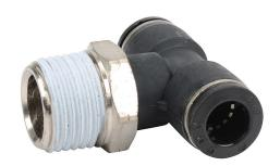
NITRA pneumatic push-to-connect fitting, male, branch tee, rotating, thermoplastic (PBT) body, nickel-plated brass threads, (2) 3/8in tube to 1/2in NPT connection(s). Package of 5.
