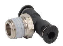
NITRA pneumatic push-to-connect fitting, branch tee, rotating, thermoplastic (PBT) body, nickel-plated brass threads, thread sealant, (1) 1/8in male NPT to (2) 1/8in push-to-connect. Package of 5.
