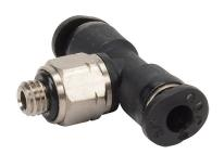
NITRA pneumatic push-to-connect fitting, branch tee, rotating, thermoplastic (PBT) body, nickel-plated brass threads, thread sealant, (1) #10-32 male UNF to (2) 1/8in push-to-connect. Package of 5.
