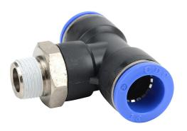
NITRA pneumatic push-to-connect fitting, branch tee, rotating, thermoplastic (PBT) body, nickel-plated brass threads, thread sealant, (1) R3/8 male BSPT to (2) 16mm push-to-connect. Package of 3.
