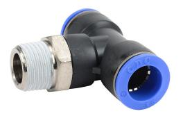
NITRA pneumatic push-to-connect fitting, branch tee, rotating, thermoplastic (PBT) body, nickel-plated brass threads, thread sealant, (1) R1/2 male BSPT to (2) 16mm push-to-connect. Package of 3.
